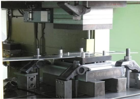
Fig. 8: Press tryout of the general blanking die
