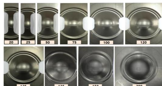
**Fig. 2: Nakajima specimens after FLD test**
