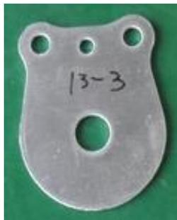
(a) Clearance 7% (b) Clearance 10% (c) Clearance 13%
