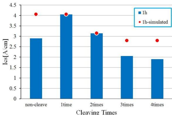
Fig. 5  $I_{cs}$  of  $\text{Al}_2\text{O}_3$  doped for 1h into the Bi-2212 single crystal
