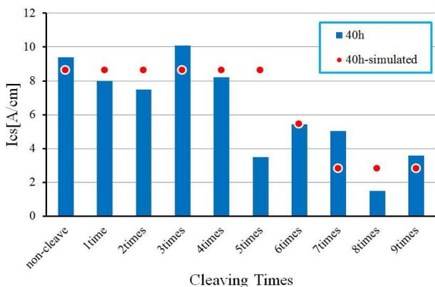
Fig. 6  $I_{cs}$  of  $\text{Al}_2\text{O}_3$  doped for 40h into the Bi-2212 single crystal
