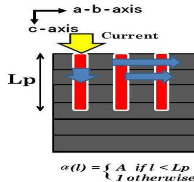
Fig.4 Model of the pinning center defused into the Bi-2212 single crystal.
