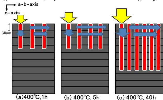
Fig.7 Model of the pinning center defused into the Bi-2212 single crystal for each times.
