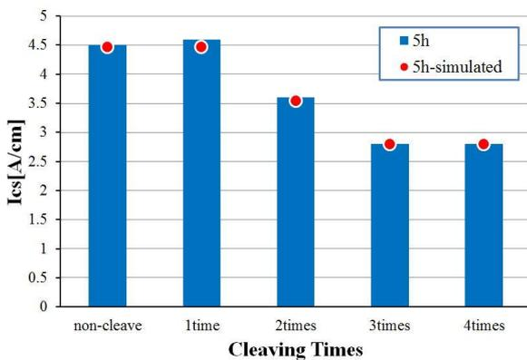
Fig.3 Ics of  $Al_2O_3$  doped for 5h into the Bi-2212 single crystal
