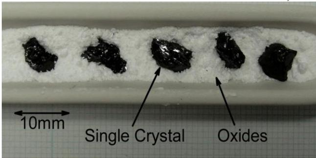
Fig.2 Photo image of Bi-2212 single crystals on the powders of oxides. The oxides were diffused into the single crystals by heat treatment.
