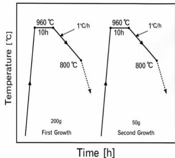
**Fig. 1 The temperature profile of Bi-2212 single crystal growth in this study**
