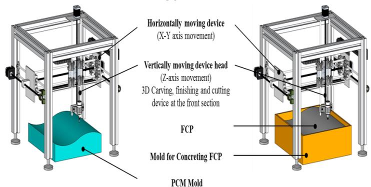
**Fig. 4: 3D Carving Machine concept**
