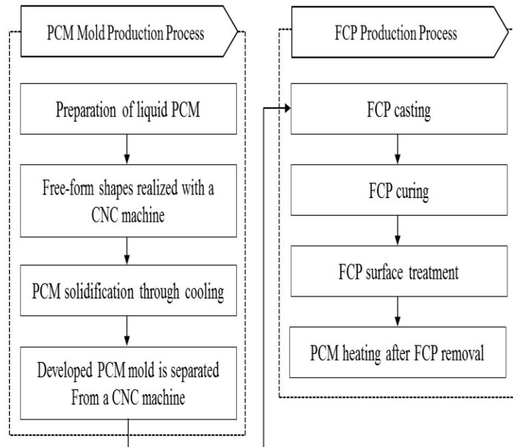
Fig. 1: Process of FCP Production Technology [11]
