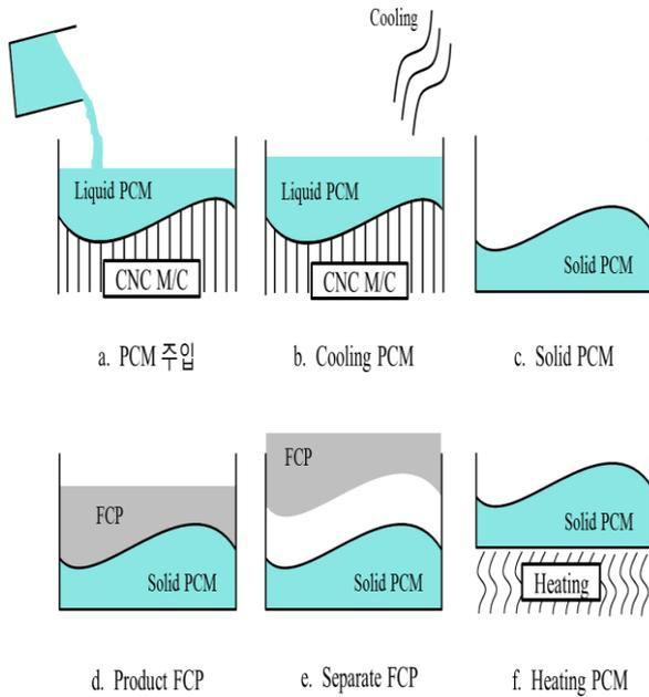
Fig. 2: PCM Mold Production Process [11]
