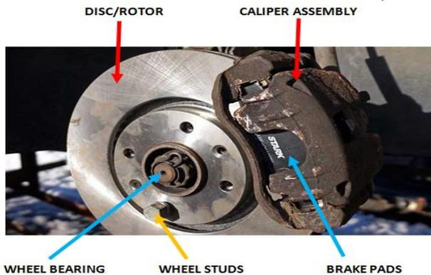
**Fig 2: Brake disc with brake pad assemble**
