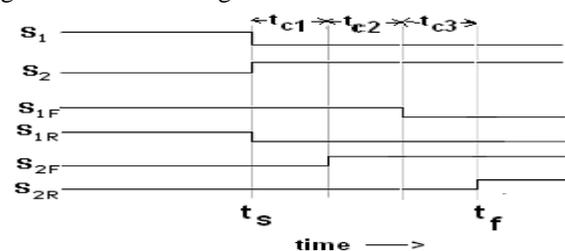
Fig. 6:- Four step current commutation
