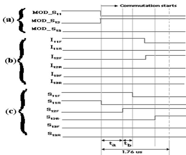
Fig.10. Commutation from S<sub>11</sub> to S<sub>12</sub> (a) Modulation signals, (b) current flow information and (c) gate signals to the IGBTs
