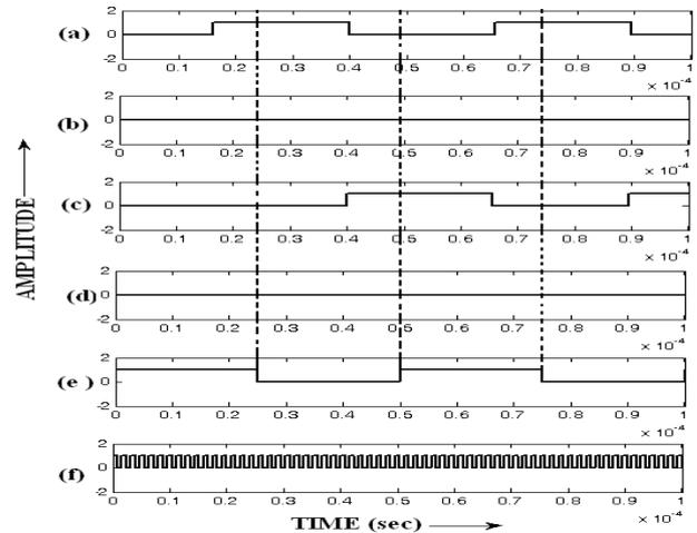
**Fig.12(b):** Three step commutation (current carrying status): (a) status signal of forward conducting IGBT (1F) in switch cell 1, (b) status signal of reverse conducting IGBT (1R) in switch cell 1, (c) status signal of forward conducting IGBT (2F) in switch cell2, (d) status signal of reverse conducting IGBT(2R) in switch cell 2, (e) Modulation signal, (f) clock input signal to the shift register
