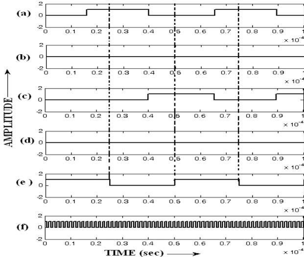
**Fig. 11(b):** Four step commutation (current carrying status): (a) status signal of forward conducting IGBT (1F) in switch cell 1, (b) status signal of reverse conducting IGBT (1R) in switch cell 1, (c) status signal of forward conducting IGBT (2F) in switch cell2, (d) status signal of reverse conducting IGBT(2R) in switch cell 2, (e) Modulation signal, (f) clock input signal to the shift register
