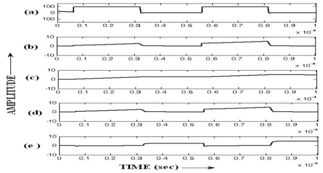
**Fig. 11(c):** Four step commutation (voltage and current in different parts): (a) Output load voltage across the R-L branch, (b) current flowing in the input supply line connected to switch cell 1, (c) current flowing in the R-L branch, (d) current flowing through Switch cell 1, (e) current flowing through switch cell 2
