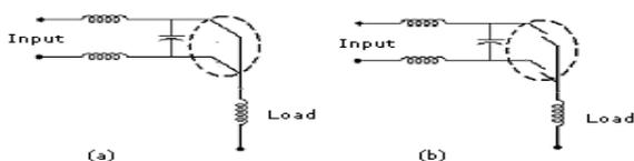
**Fig. 3. Unwanted switching: (a) short circuit at input lines (b) open circuit at output lines**
