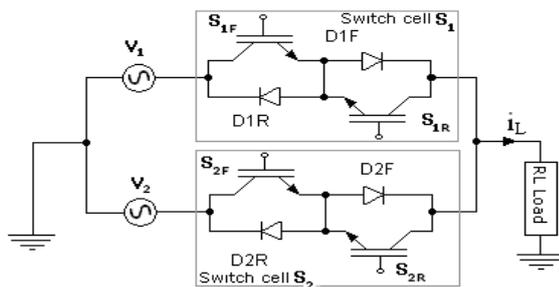
Fig.5. Two phase to single phase matrix converter considered in the scheme.
