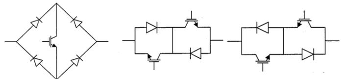
**Fig. 2.** Realization of bi-directional switch (a) diode bridge with single IGBT, (b) common collector configuration, (c) common emitter configuration
