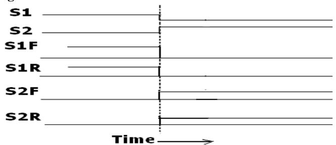
Fig. 8 Single step current commutation
