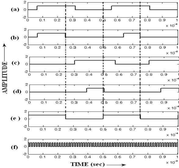
**Fig.11(a).** Four step commutation: Gating pulses (a) gate signal for the outgoing IGBT 1F in switch cell1, (b) gate signal for the outgoing IGBT 1R in switch cell 1, (c) gate signal for the incoming IGBT 2F in switch cell2, (d) gate signal for the incoming IGBT 2R in switch cell2 and (e) modulation signal for the switch cell 1, (f) clock input for the shift register]=
