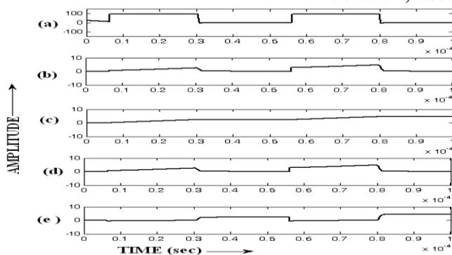
**Fig.12 (c): Three step commutation (voltage and current in different parts): (a) Output load voltage across the R-L branch, (b) current flowing in the input supply line connected to switch cell 1, (c) current flowing in the R-L branch, (d) current flowing through Switch cell 1, (e) current flowing through Switch cell 2**
