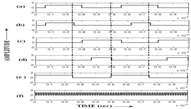
**Fig. 12(a).** Three step commutation: Gating pulses (a) gate signal for the outgoing IGBT 1F in switch cell1, (b) gate signal for the outgoing IGBT 1R in switch cell 1, (c) gate signal for the incoming IGBT 2F in switch cell 2, (d) gate signal for the incoming IGBT 2R in switch cell2 and (e) modulation signal for the switch cell 1, (f) clock input for the shift register
