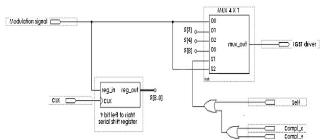
Fig. 9 Control logic for commutation of a single IGBT switch.
