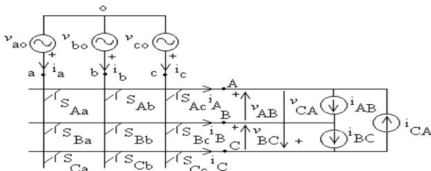
**Fig.1.**Matrix converter circuit
