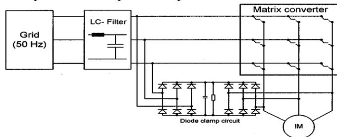
**Fig. 4. Matrix converter with clamp circuit**
