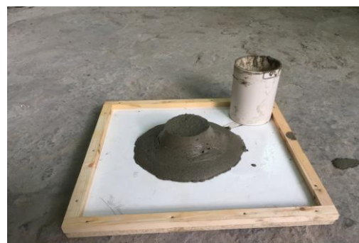
Fig 3: Spread ability test
