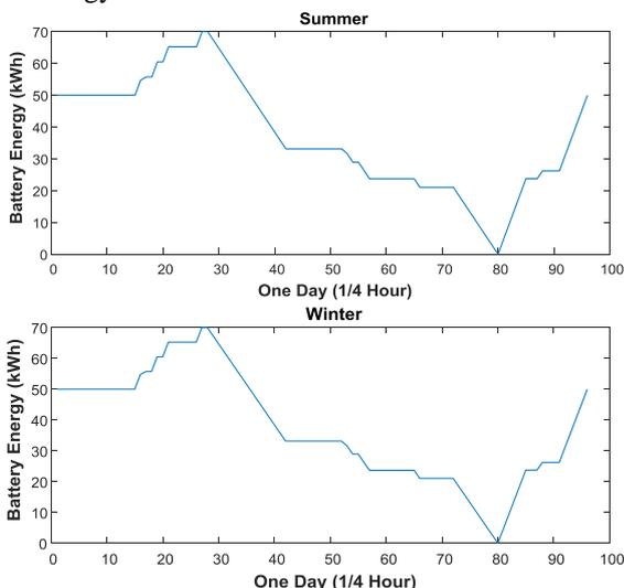
**Fig.5. BESS Charge/Discharge in One-day Cycle**
