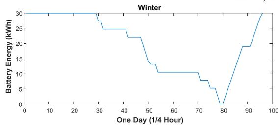
Fig.7. BESS Charge/Discharge after Peak Shaving
