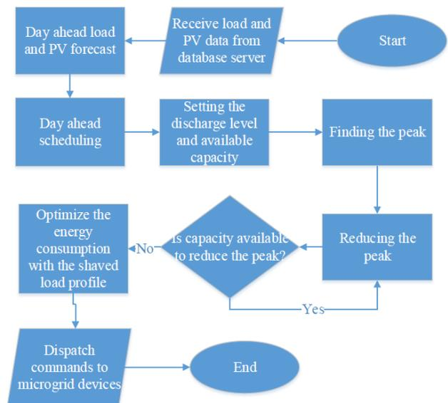
Fig.2. Scheduling System Including Peak Shaving Algorithm
