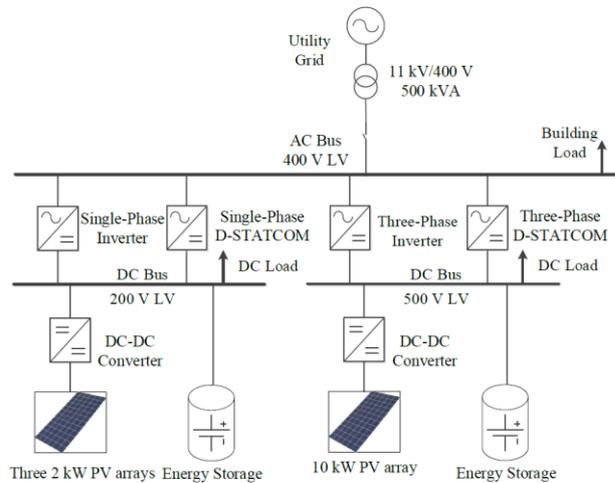
Fig.3. Experimental Microgrid Structure
