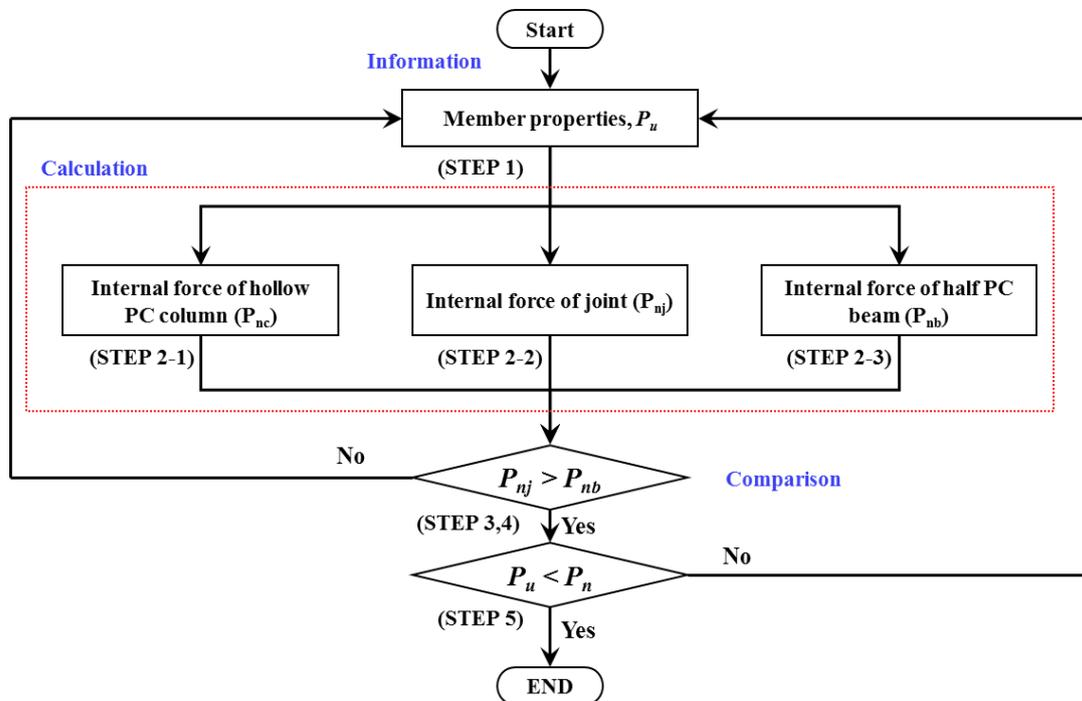
Fig 3 Design procedure of the joint using HPC column
