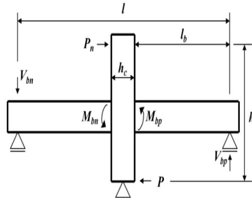
Fig 4 Interior beam-column joint
