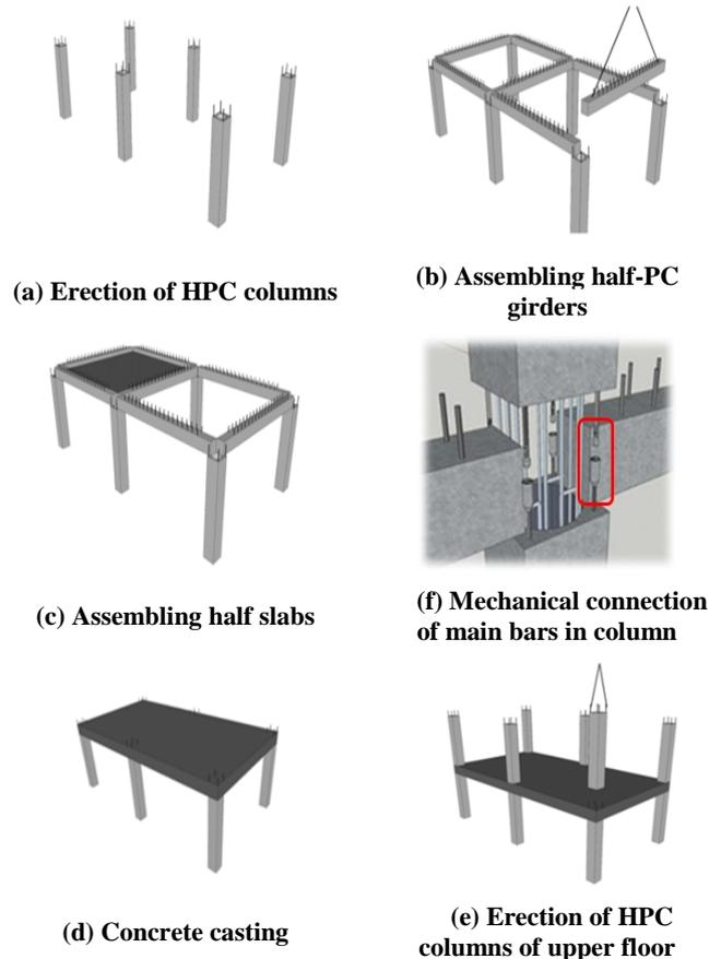
**Fig. 1** Construction process of PC frame system with HPC columns
