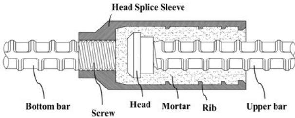
Fig. 2 Shape and detail of head-splice sleeve (HSS)
