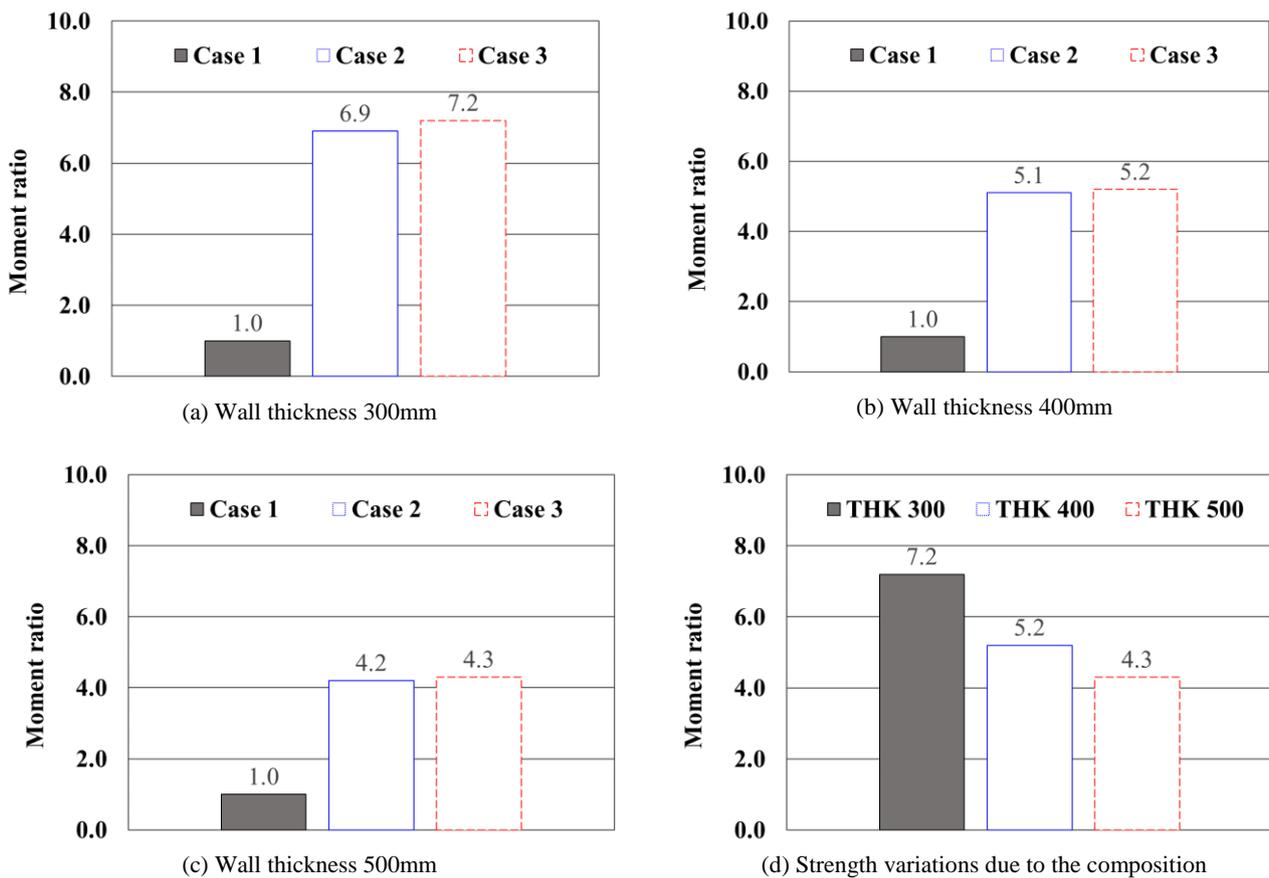
Fig. 6: Composite effect of walls with same magnitude of vertical reinforcement
