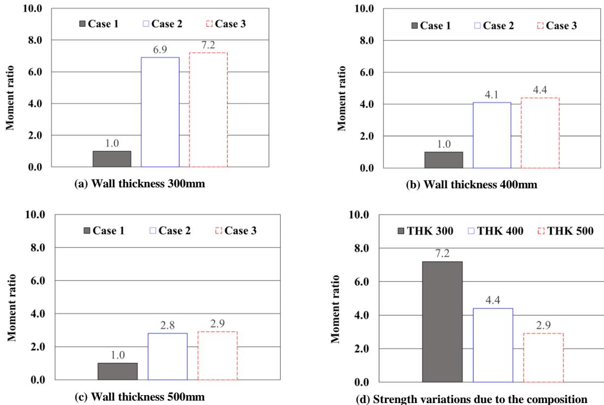
Fig. 7: Composite effect of walls with same ratio of vertical reinforcement
