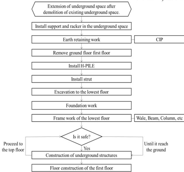
Fig. 1: Flow chart of underground extension
