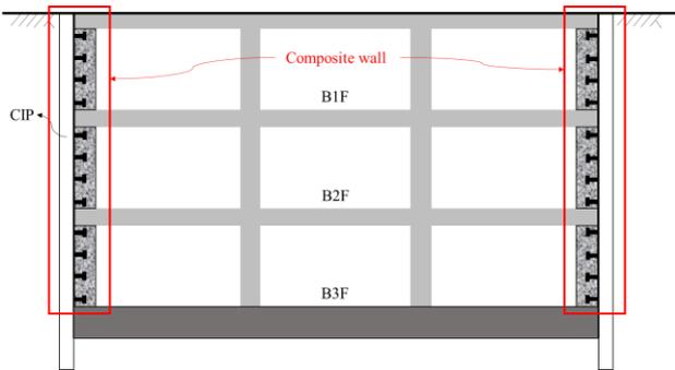
Fig. 2: Underground structure with composite wall
