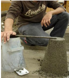
Plate 2: Slump test being conducted on the concrete sample with 100% steel slag [4]
