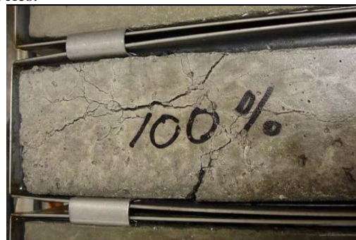
Plate 5: 100% A steel slag specimen with no air entraining admixtures under the freeze-thaw machine
