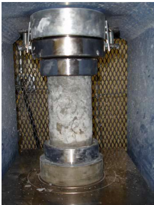
Plate 3: Shows the Compression test conducted on a concrete specimen with steel slag aggregates [2]
