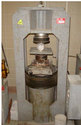
Plate 4: Splitting tensile Test conducted on concrete specimen [2]
