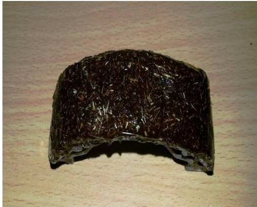
Fig 10 Brake pad made up of sample 1 composition
