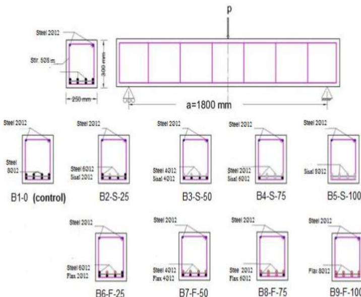
Fig. 2 Details of tested beams
