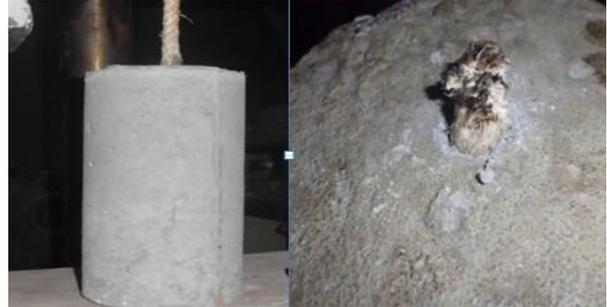
Fig. 3 Bond Failure after Test
