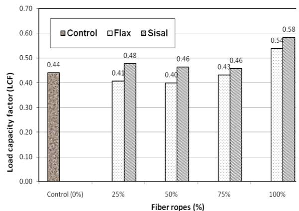
**Fig. 13 Load Capacity Factor (LCF) of Tested Beams**
