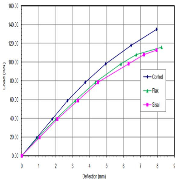
**Fig. 5 Load-deflection relationship of beams reinforced with (75% steel + 25% fiber rope)**
