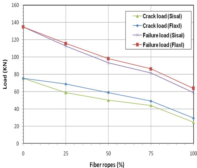
**Fig. 11 Cracking and failure loads of tested beams**
