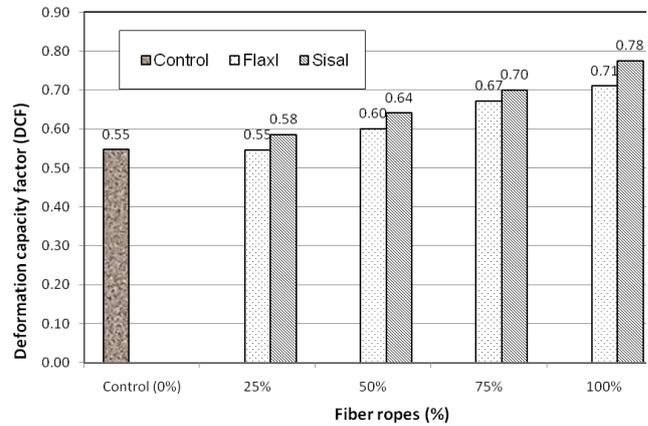
**Fig. 12 Deformation Capacity Factor (DCF) of tested beams**
