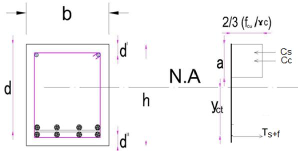
Fig. 4 Acting Forces on the Cross Section Area of Tested Beam
