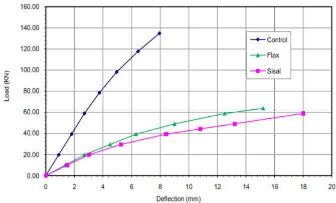
**Fig. 8 Load-deflection relationship of beams reinforced with (0% steel +100% fiber rope)**
