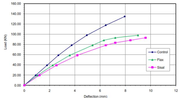
**Fig. 6 Load-deflection relationship of beams reinforced with (50% steel + 50% fiber rope)**
