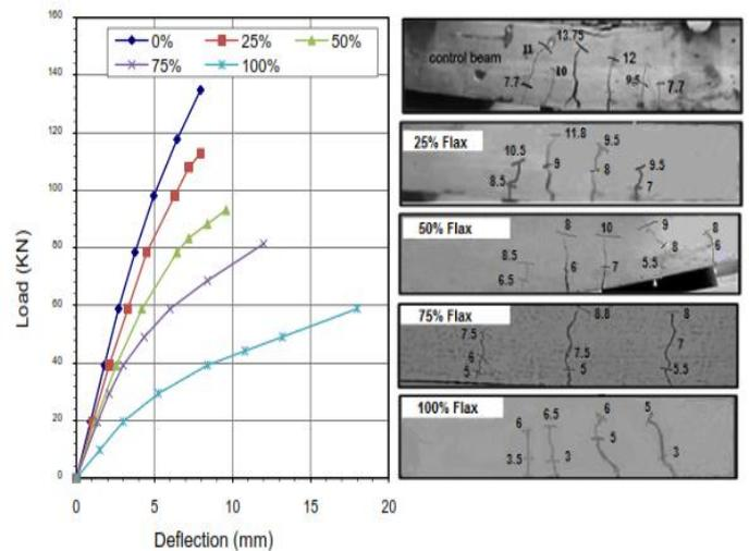
**Fig. 9 Load-deflection of beams reinforced with flax bars and cracking pattern for tested beams**
