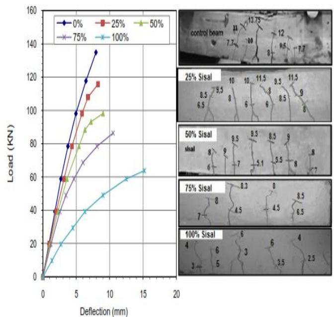
**Fig. 10 Load-deflection of beams reinforced with sisal bars and cracking pattern for tested beams**
