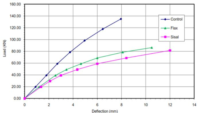
**Fig. 7 Load-deflection relationship of beams reinforced with (25% steel + 75% fiber rope)**
