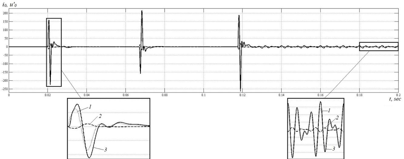
**Fig. 1. Phase relationships of zero-sequence currents  $i_0$  in damaged and undamaged connections (1 and 2) and zero-sequence voltage derivative  $u'_0$  (3) in SPEF transient and steady-state modes**
