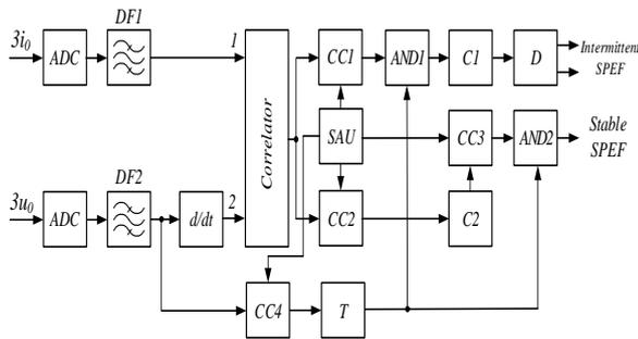
**Fig. 2. Structural diagram of universal directional protection against SPEF based on HH for compensated MV cable networks**
