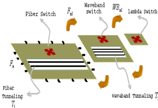
Fig. 4 Internal Architecture of the MG-OXC with Nodal Degree of 4
