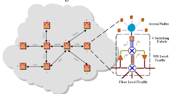
Fig. 3 Illustrates the Switching and, Tunneling, and Grooming Levels of the MG-OXC
