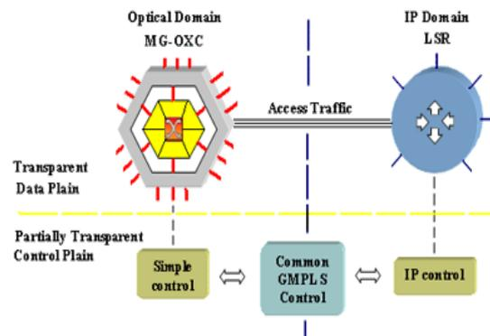
Fig. 2 GMPLS Based Control Plane Running over MG-OXC
