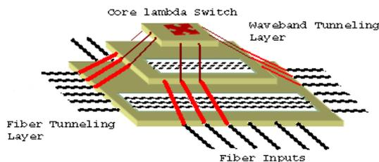
Fig. 1 Illustrates the Architecture of the MG-OXC
