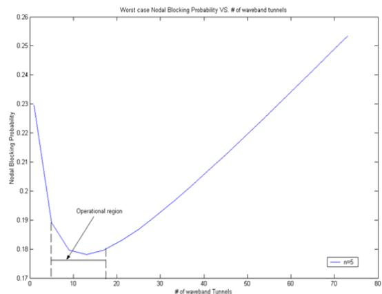
Fig. 9 Effects of Waveband Tunnels on Blocking Probability
