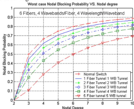
Fig. 6 Nodal Blocking Probability vs. Nodal degree for MG-OXC
