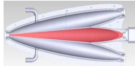
Fig. 6. Inner shapes of optical waveguide with three ellipsoidal paths
