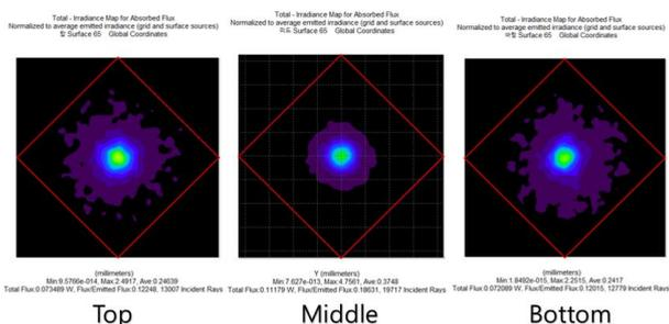
Fig. 7 Simulation results of absorbed energy pattern at three regions in the ellipsoidal structure
