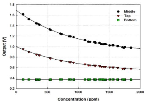
Fig. 8 Output voltages of infrared sensors located at three focal points in ellipsoidal structure
