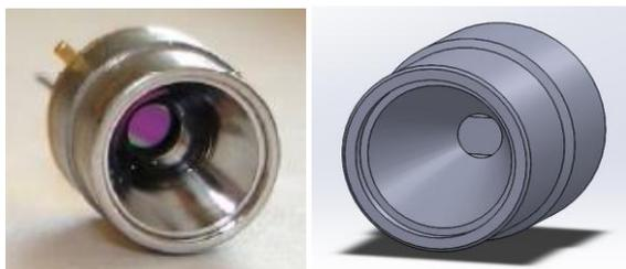
**Fig. 1. A 3-D shape to model blackbody infrared source(MIRL17-900)**
