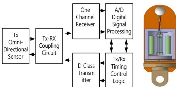
Fig. 3 Functional block of pinger system
