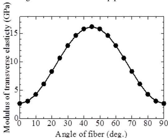
Fig. 8: Modulus of transverse elasticity of pipe structure
