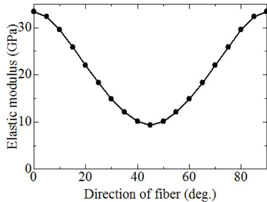
Fig. 5: Elastic modulus vs. direction of fiber
