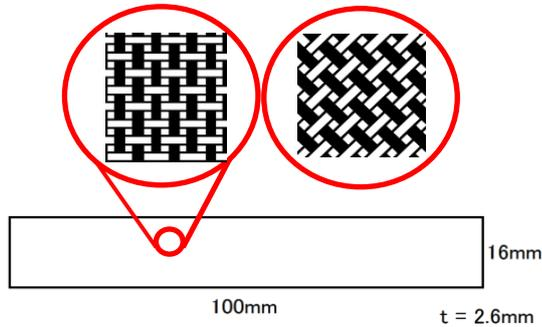
Fig. 2: Fiber direction and dimension of specimen
