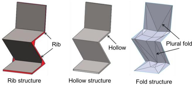
Fig. 15: Three kinds of CFRP structural models
