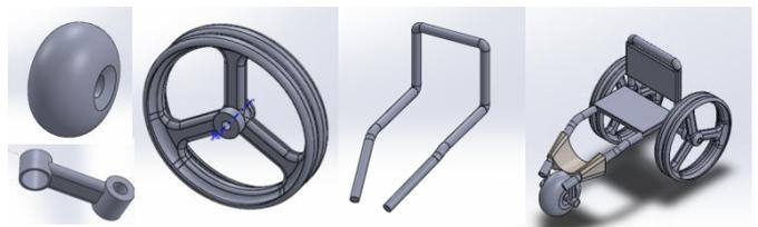
Fig. 9: CAD model of parts and assembled wheelchair
