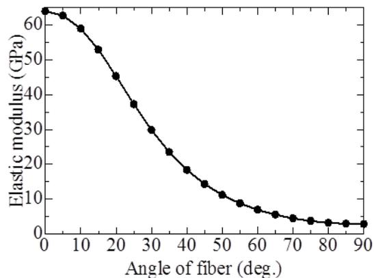
Fig. 6: Elastic modulus vs. angle of fiber
