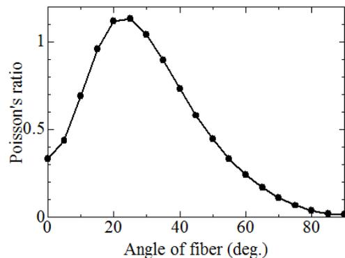
Fig. 14: Poisson's ratio of CFRP structure
