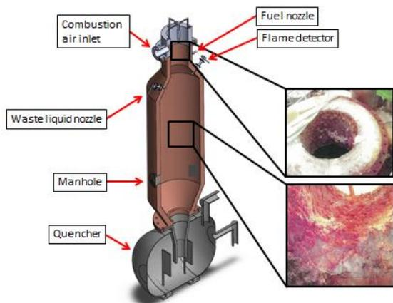
Fig. 1: Incinerator
