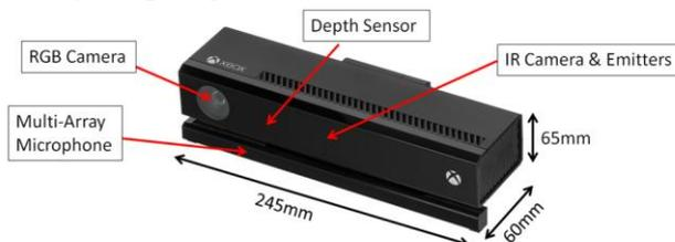
Fig. 3: Kinect sensor
