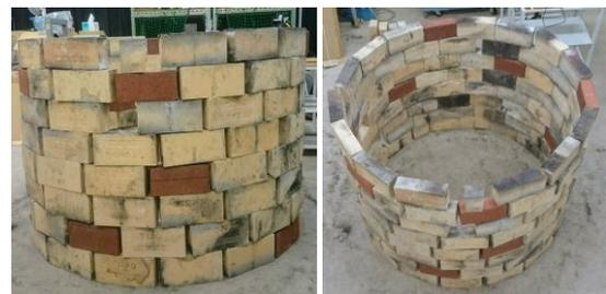
Fig. 15: Pseudo model of incinerator
