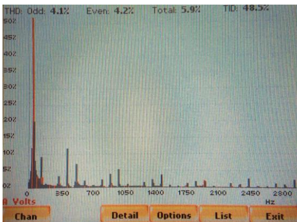
Fig. 20 Total Harmonic Distortion (THD) with linear load
