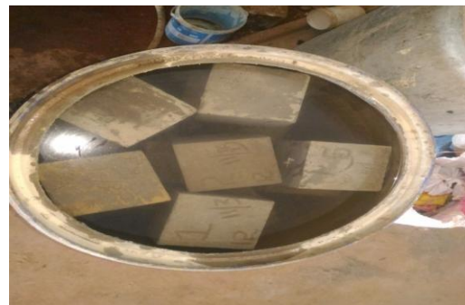
FIG -2: CURING OF CUBES
