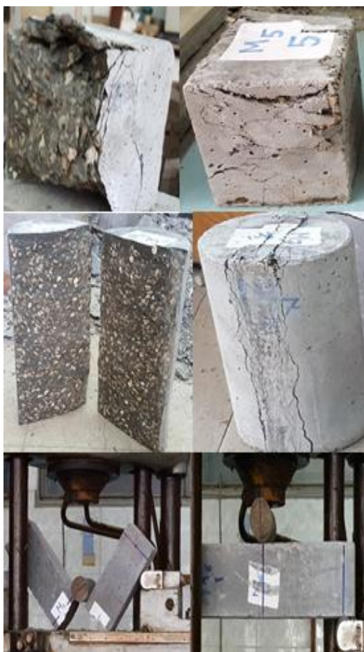
Fig. 10 Failure modes of the concrete mixes under various loading (right with fiber and left without fiber).
