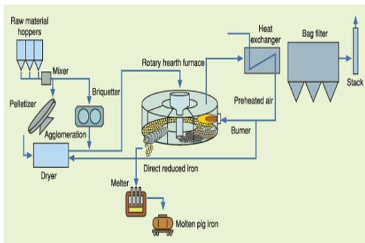
Fig 7: Line Diagram of Rotary Hearth Furnace
