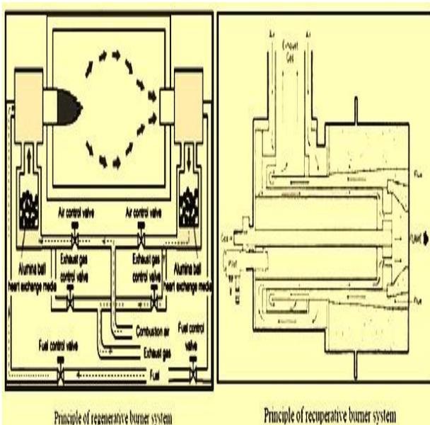
Fig 13: Principle of Regenerative and Recuperative Burner
