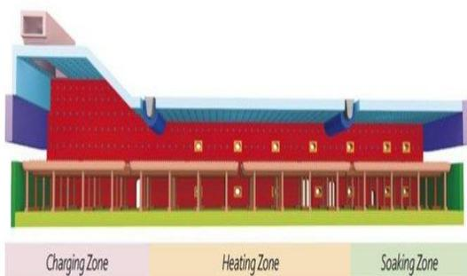
Fig 4: Zones of Reheating Furnace
