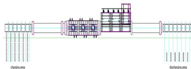
Fig 10: Line Diagram of Roller Hearth Furnace
