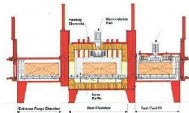
Fig 5: Batch Furnace
