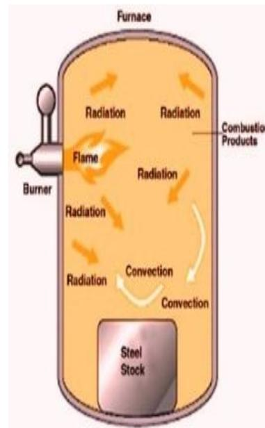
Fig 2: Reheating Furnace
