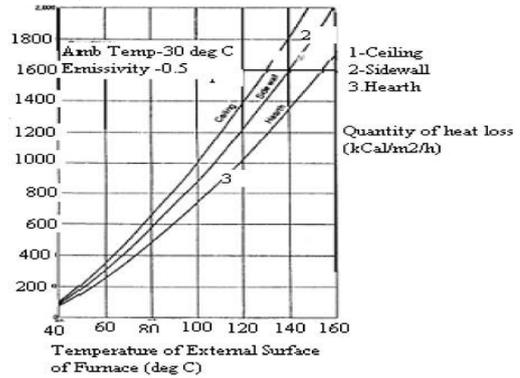
Fig 15: Quantity of Heat Release at Various Temperatures
