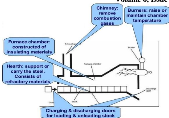
Fig 3: Components of Reheating Furnace
