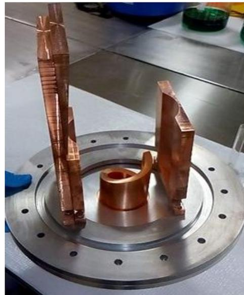
**Fig.7 Quasi optical mirrors system of Gyrotron**
