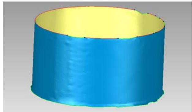
Fig 10 The tank's mesh creation by the total station scanning.
