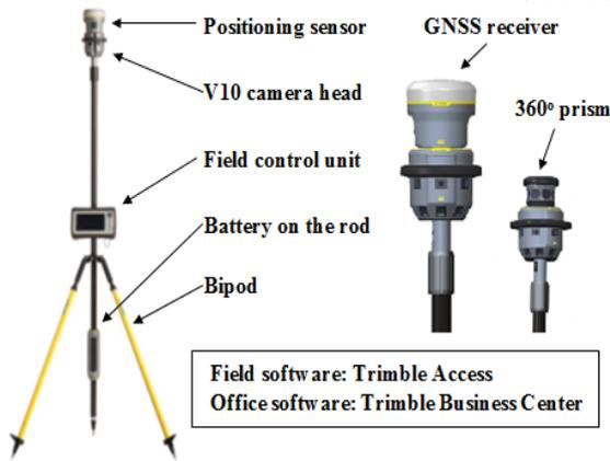
Fig 1: The components of V10 Imaging Rover
