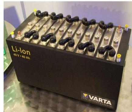
Fig.3. A hybrid car battery
