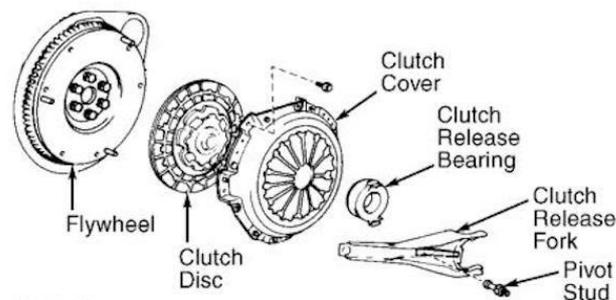
Fig 1: Basic Diagram of Clutch System
