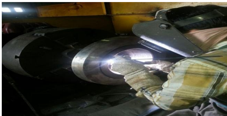
Fig: 2 Specimen for abrasive wear with colmonoy 4 coating/welding in industry
