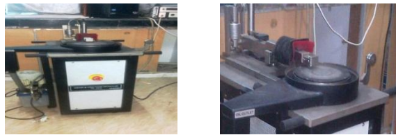
Fig: 3, Machine for conducting wear test (pin on disc wear testing machine)
