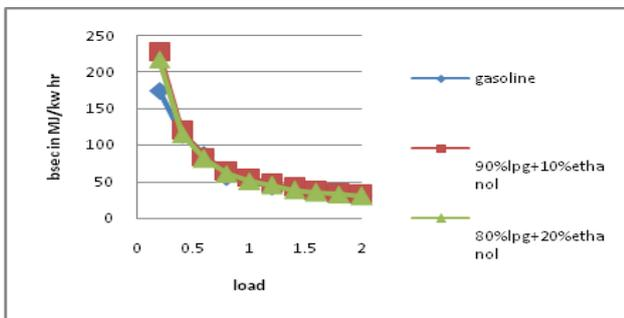
Fig 2. Brake specific energy consumption at compression ratio 11.
