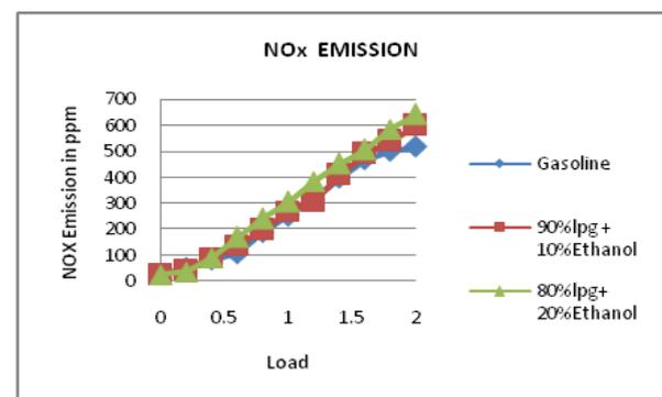
Fig 12. NO<sub>x</sub> Emission at compression ratio 11.
