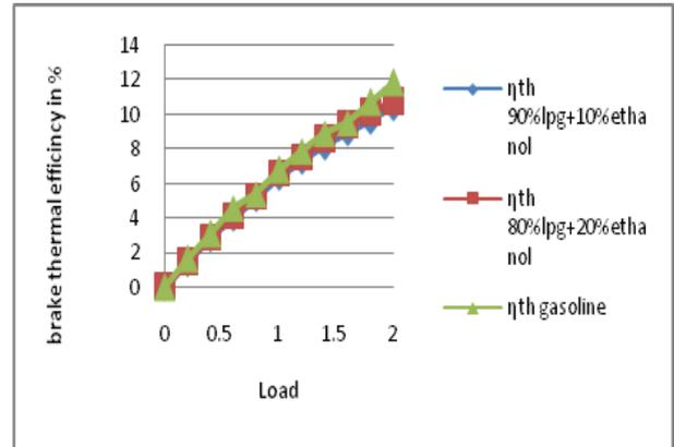
Fig 3. Brake thermal efficiency at compression ratio 10
