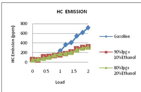
Fig 8. HC Emission at compression ratio 11.
