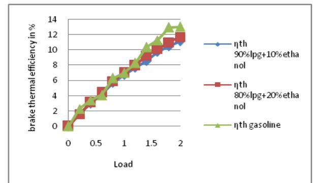
Fig 4. Brake thermal efficiency at compression ratio 11
