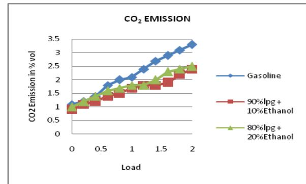
Fig 10. CO<sub>2</sub> Emission at compression ratio 11.
