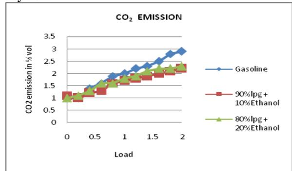
Fig 9. CO<sub>2</sub> Emission at compression ratio 10.
