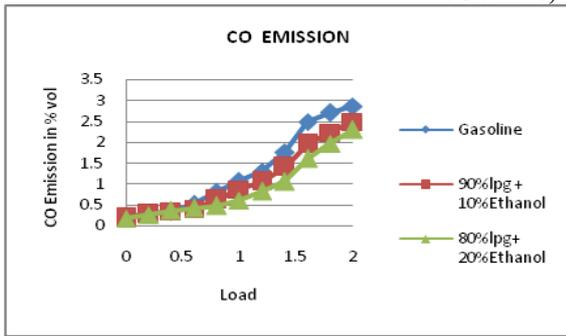
Fig 6. CO Emission at compression ratio 10.
