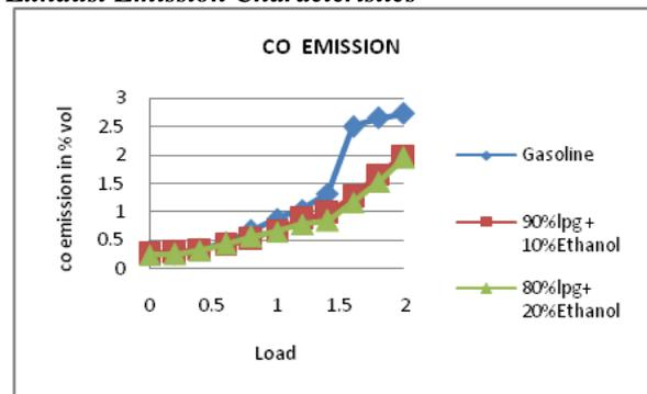
Fig 5. CO Emission at compression ratio 10.
