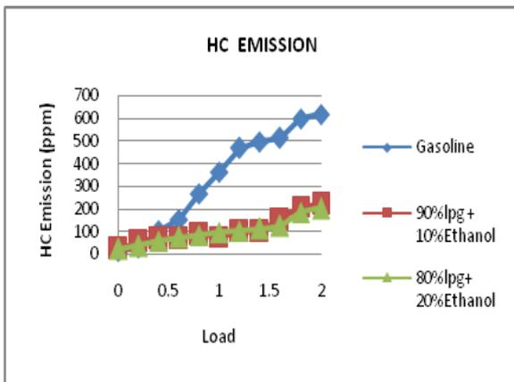
Fig 7. HC Emission at compression ratio 10.
