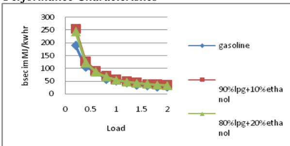
Fig 1. Brake specific energy consumption at compression ratio 10.
