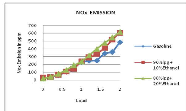
Fig 11. NO<sub>x</sub> Emission at compression ratio 10.
