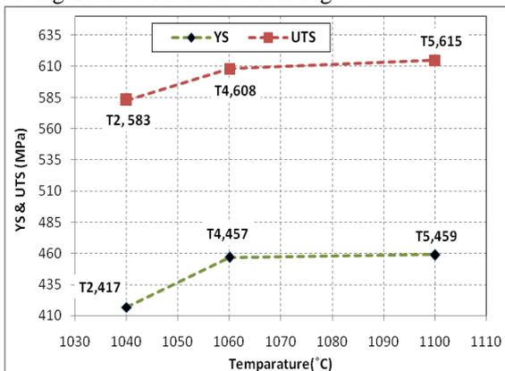
Fig.6: Effect of temperature on YS & UTS
