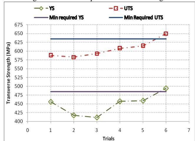
Fig. 3: Bend YS & UTS in Transverse Direction.
