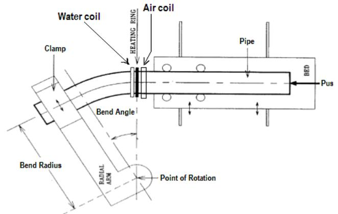
Fig. 1: Line diagram of hot induction bending process
