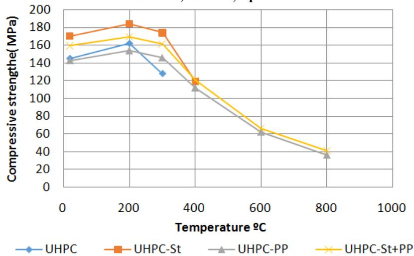
Fig.2. Residual compressive strength of UHPC mixes with increasing temperature
