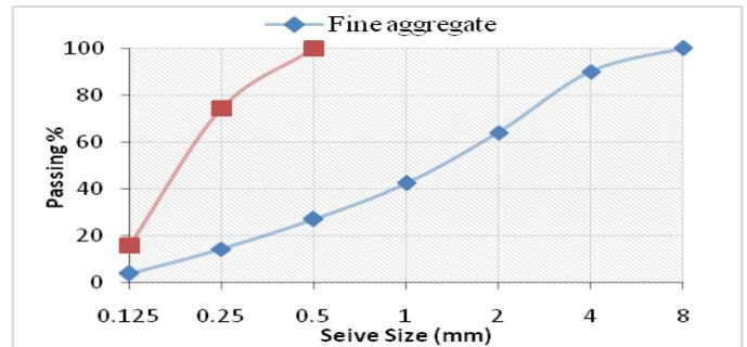
Fig. 1 Grading curves of fine sand and fine aggregates
