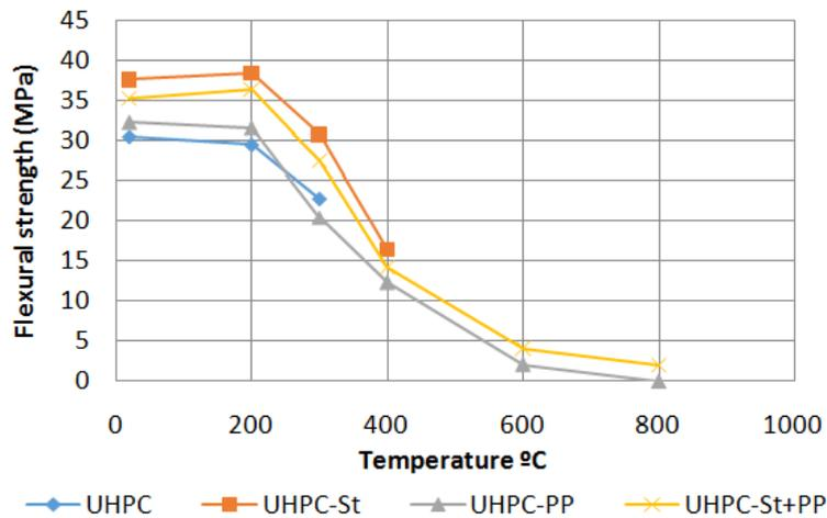
Fig. 5. Residual flexural strength of UHPC mixes with increasing temperatures
