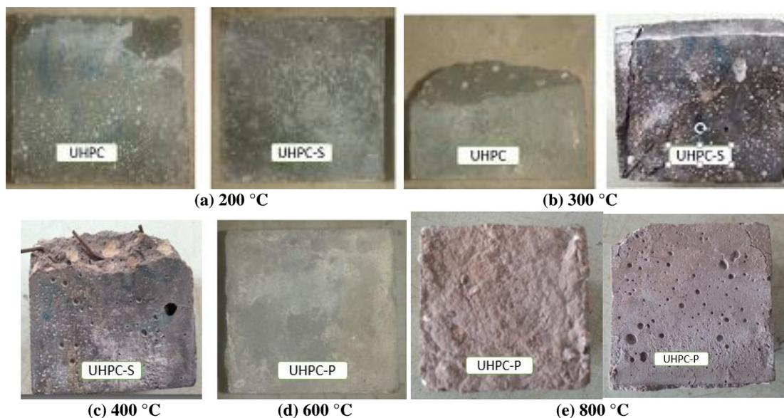
Fig.4 Spalling and Surface character of UHPC and UHPFRCs at elevated temperatures
