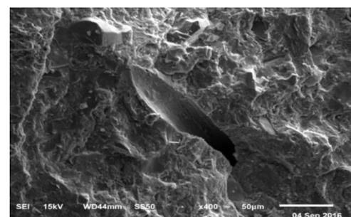
Fig.3 Void left by melting Polypropylene fiber in UHPC-PP Matrix
