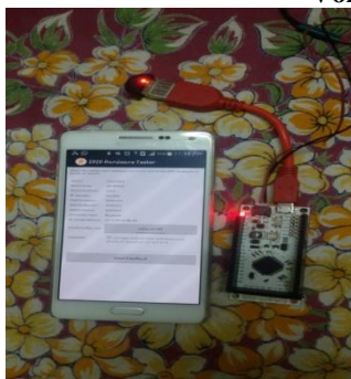
Fig.9 LED off when it is Unpaired
