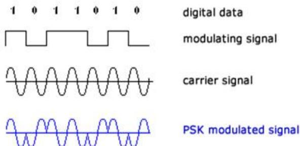
Fig.6 Shows PSK modulation technique. A digital data 1011010 and a carrier signal which after modulation gives a PSK modulated signal.
