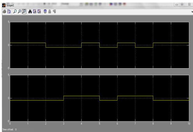
Fig.15 Scope output 1 of QPSK which shows two signals coming from two NRZ blocks.
