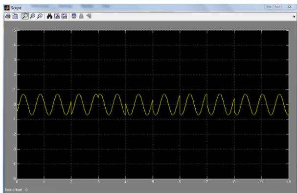
Fig.14 scope output of QPSK which is product of two blocks whose phase is 0 radian and pi/2 respectively with frequency 10 rad/sec and amplitude 1
