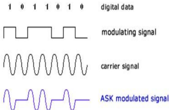
Fig.4 Shows ASK modulation technique in which a digital data 1011010 is to be transmitted using ASK modulation
