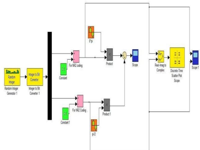
**Fig.11 shows implementation of QPSK using MATLAB Simulink. Output signal is plotted on discrete time scatter plot as shown in figure.**
