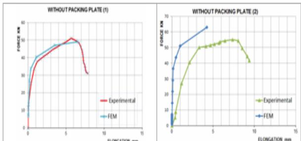
Fig.11: Validation of Relation between Elongation and Force for Specimen (1)
