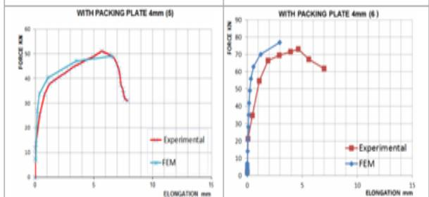
Fig.15: Validation of Relation between Elongation and Force for Specimen (5)
