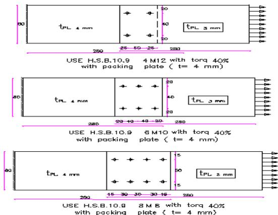
**Fig.23: Specimen Geometry in Case of Change Number of Bolts with the Same Area of Bolts.**
