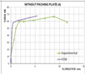
Fig.14: Validation of Relation between Elongation and Force for Specimen (4)
