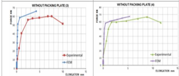
Fig.13: Validation of Relation between Elongation and Force for Specimen (3)
