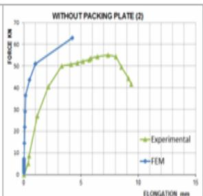
Fig.12: Validation of Relation between Elongation and Force for Specimen (2)
