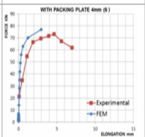
Fig.16: Validation of Relation between Elongation and Force for Specimen (6)
