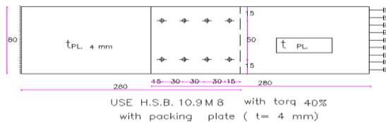
**Fig.24: Specimen Geometry in Case of Study the Effect of Plate Thickness (using 8M8).**
