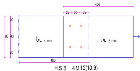
Fig.8: Specimen Geometry
