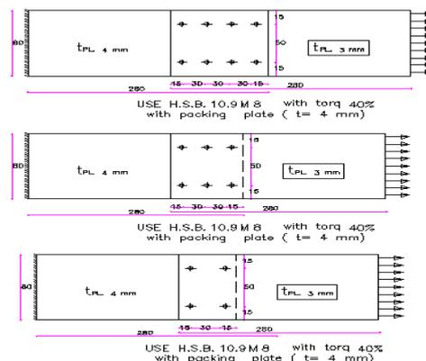
**Fig.25: Specimen Geometry in Case of Study the Effect of the Bearing Stress Distribution with Different Number of H.S Bolt having the Same Diameter.**
