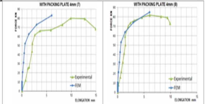
Fig.17: Validation of Relation between Elongation and Force for Specimen (7)
