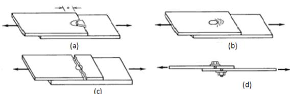
Fig. 2: Types of Failure of Bolted Connections
