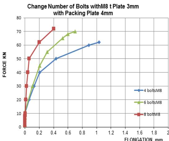
Fig. 32: Relation between Axial Force and Elongation in Case of Change Number Bolts.
