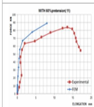
Fig.21: Validation of Relation between Elongation and Force for Specimen (11)
