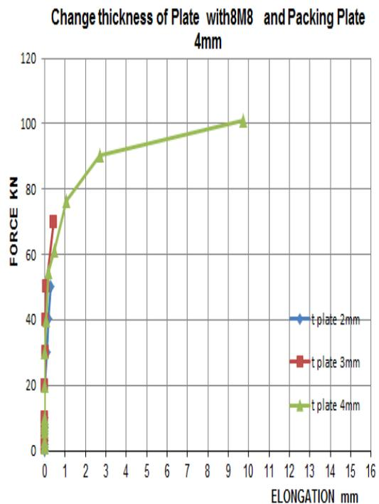
Fig. 28: Relation between Axial Force and Elongation in Case of Change plate thickness (using 8M8).
