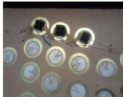
Fig. 2 series connected pressure sensors
