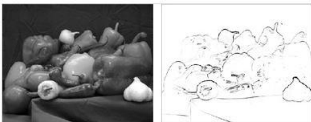
Fig.3 Image segmentation using Fuzzy Logic method [33]
