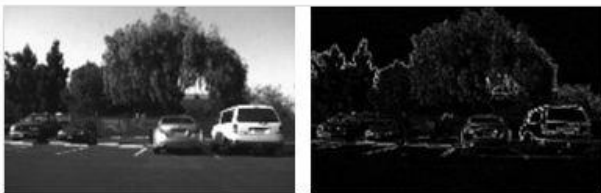
Fig.1 Image segmentation using Sobel method [32]
