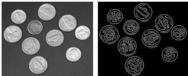
Fig.2 Image segmentation using Canny method [32]
