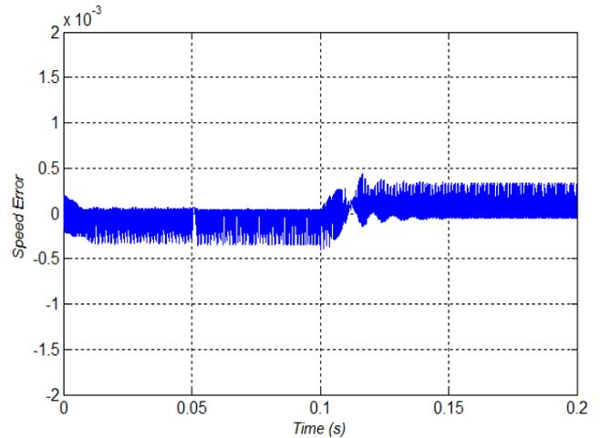
**Fig 5 :The error between estimated and actual speed**
