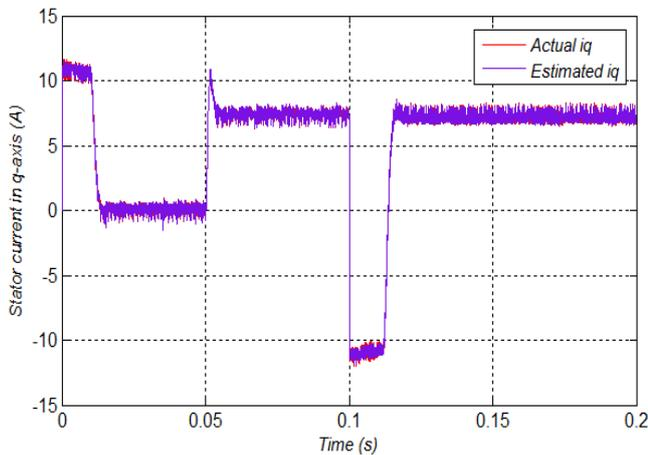
Fig 9: Estimated and actual current in q-axis
