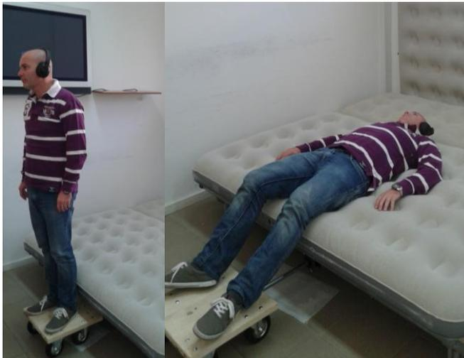
Fig. 4. Movable Platform for fall events simulation.
