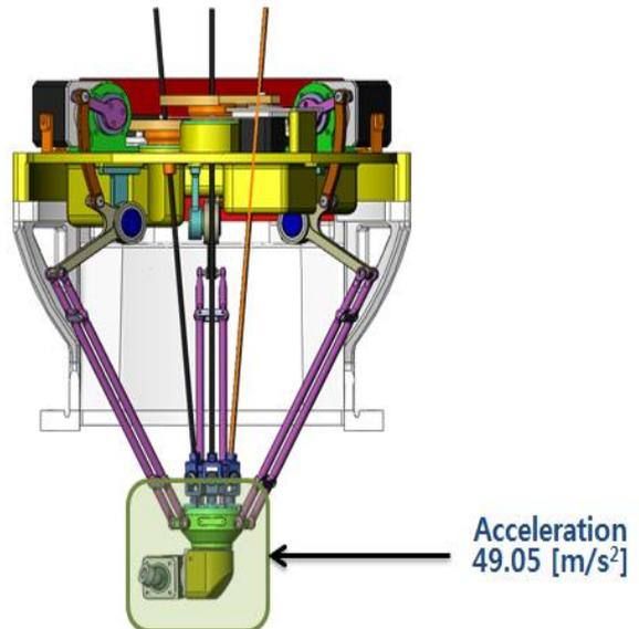
Fig. 16 The moving platform under the maximum acceleration
