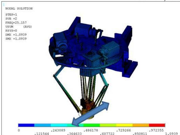
Fig. 14 Mode shape: 2<sup>nd</sup> mode (25Hz)
