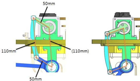
Fig. 3 Parallelogram of hinge arm assembly
