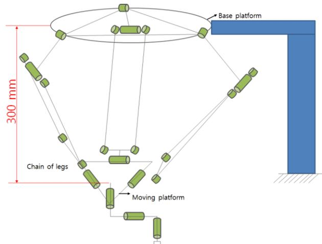
Fig. 1 Kinematic diagram of the parallel kinematic robot
