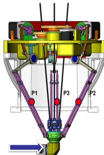
Fig. 17 Excitation location & vibration measurement position
