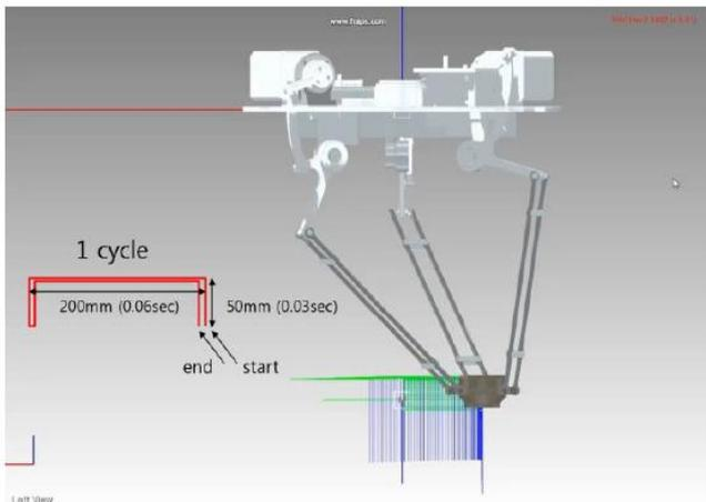
**Fig. 9** The developed dynamic simulation tool
