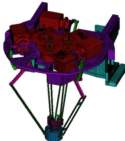
**Fig. 12** FEM modeling of the parallel kinematic robot
