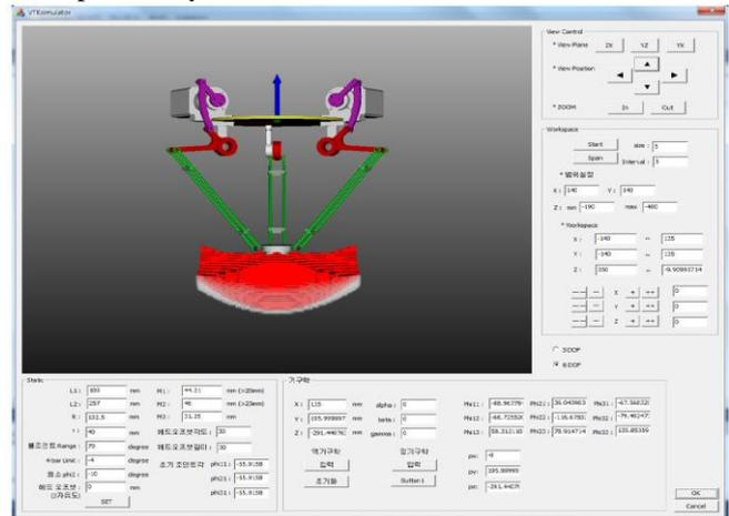
Fig. 7 Developed workspace analysis tool
