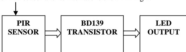
Fig 2: Block diagram of PIR sensor
