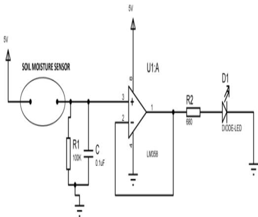
**Fig 4 Circuit diagram of soil moisture sensor**
