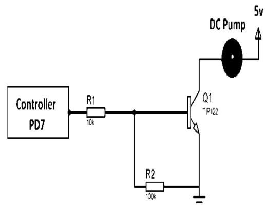
**Fig 6: Circuit diagram of DC pump**
