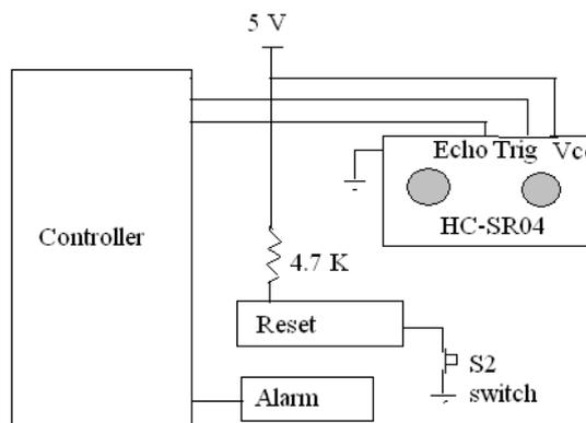
**Fig 6: Circuit diagram showing interfacing of level sensor.**
