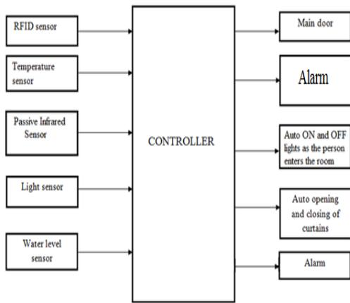
Fig. 1: Block diagram of sensor network interface to microcontroller in home automation system.
