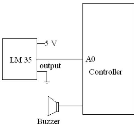
**Fig 4: Interfacing of LM35 sensor with Arduino.**
