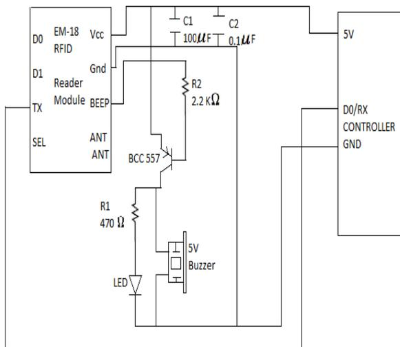
Fig 2: Interfacing EM-18 RFID reader with Arduino.
