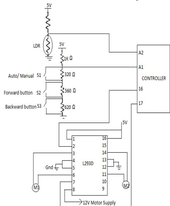
Fig 3: Circuit diagram of LDR interface in automatic curtain controller.
