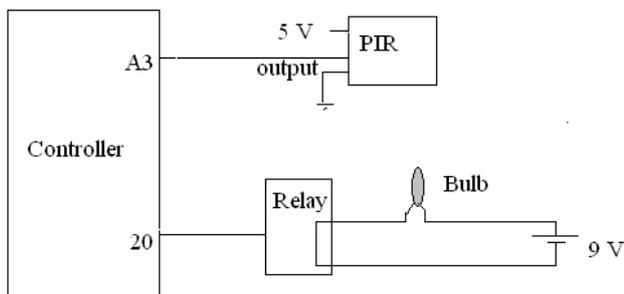
**Fig 5: Circuit diagram of PIR Sensor interface.**
