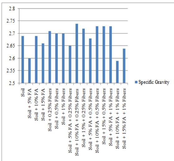
Fig.5. Results of Specific gravity test
