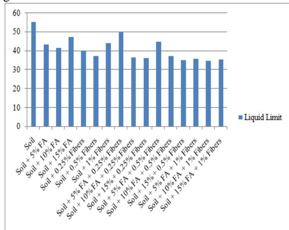
Fig. 7. Results of liquid limit test
