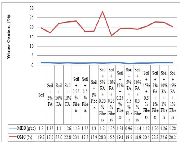
Fig. 11. MDD v/s OMC for Soil + % Fly ash + % Fibers
