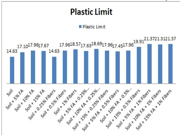
Fig. 9. Results of plastic limit test
