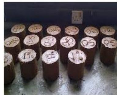
**Fig.4. Samples of Unconfined compression test**
