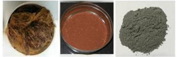
**Fig. 1. Samples of (b) lateritic soil, (a) coir fiber and (c) fly ash**
