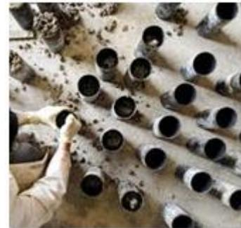
**Fig.3. Sample preparation for compaction test**
