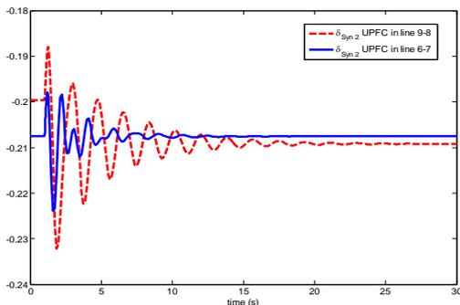
Fig 5: comparison between damping of angle oscillations of generators by replacement of UPFC in line 8-9 and 6-7
