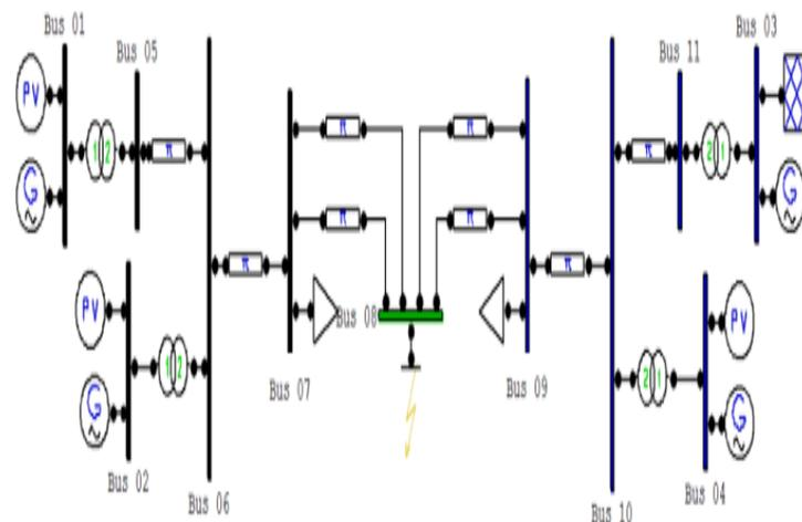
Fig 3: 11-bus system 4 car IEEE standard
