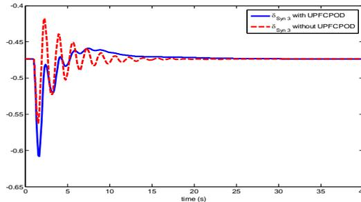
Fig (7): the damping of rotor angle oscillations of generators (8 syn3) system 11 BUS in the state Without UPFC and UPFCPOD
