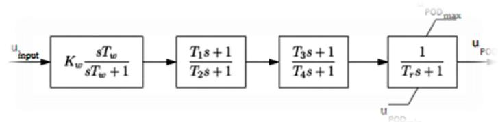
Fig 2: depiction of diagram of POD controller
