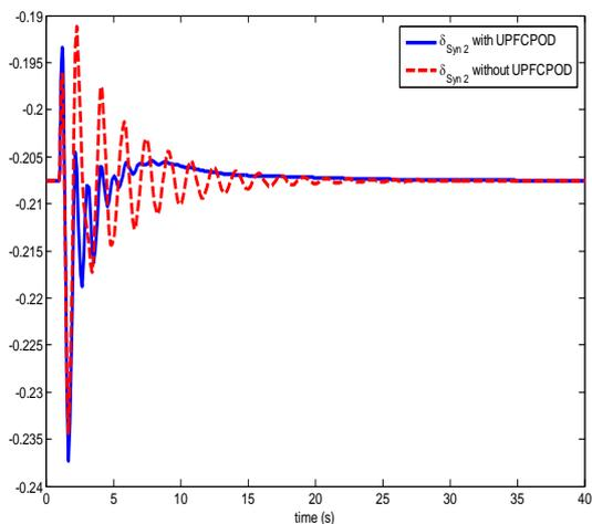
Fig 6: the damping of rotor angle oscillations of Generator 2 (6 syn) system 11 BUS in the state without UPFC AND UPFCPOD.
