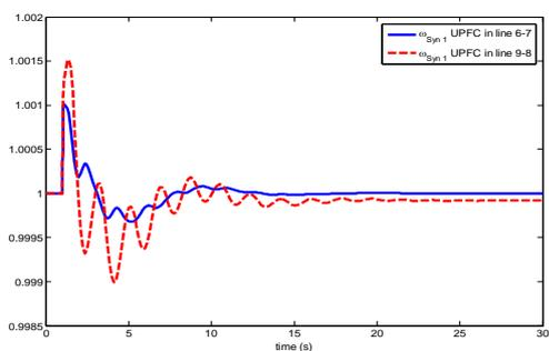
Fig 6: Comparison between damping of velocity oscillations of generator by replacement of UPFC in line 8-9 and line 6-7
