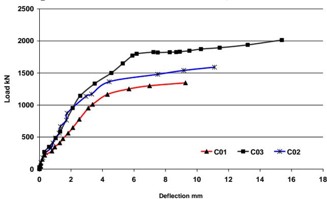
Fig 8 Load-deflection of columns C01, C02 and C03
