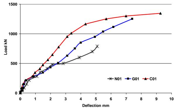
Fig. 4 Load-deflection of columns N01, G01 and C01
