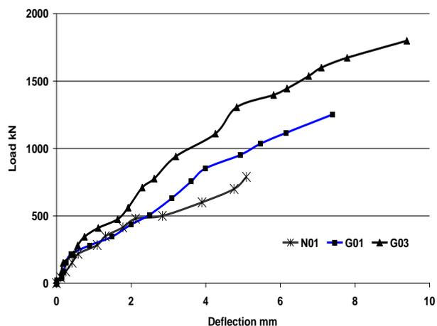
Fig 6 Load-deflection of columns N01, G01 and G03
