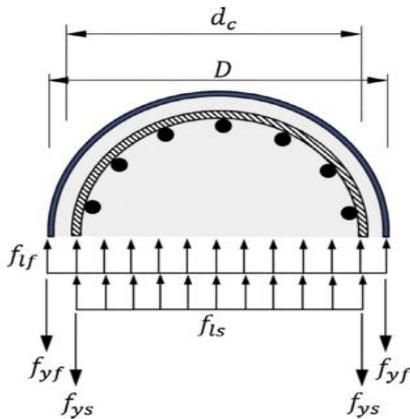
Fig. 10 Confining mechanism for concrete confined by FRP and steel [18].
