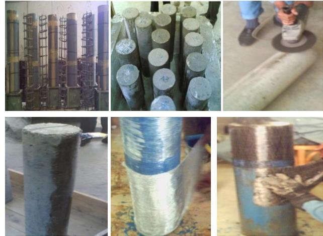
Fig. 1 Fixing column with FRP
