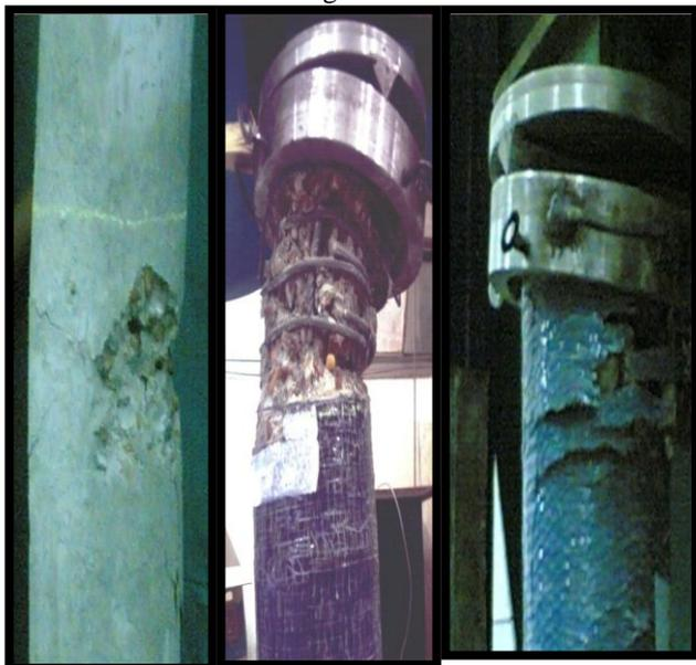
Fig. 9 Mode of failure for columns under eccentric load
