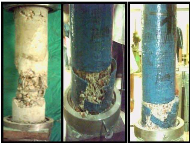
Fig. 3 Mode of failure for columns under concentric load
