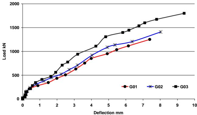
Fig 7 Load-deflection of columns G01, G02 and G03
