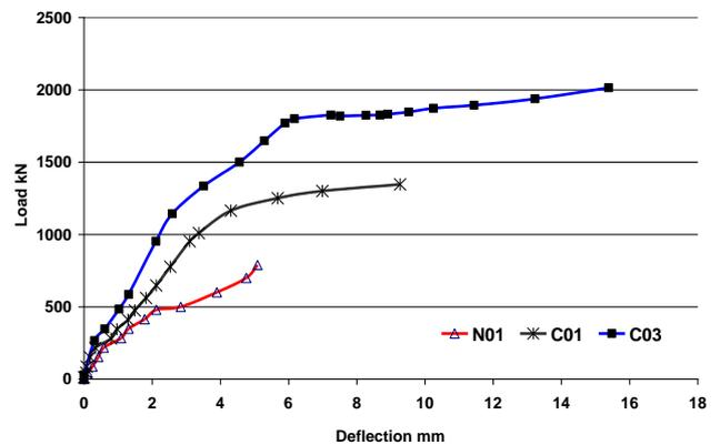
Fig. 5 Load-deflection of columns N01, C01 and C03
