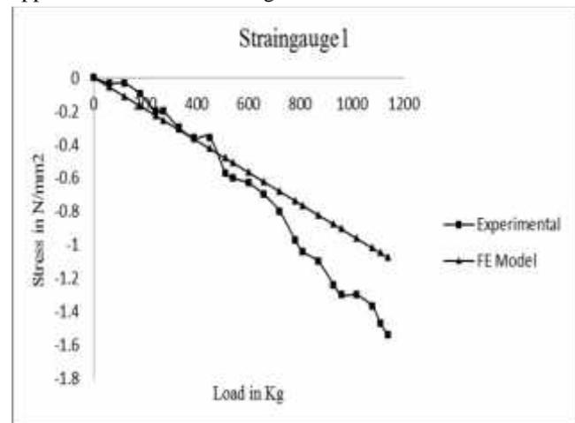
Fig.18. Stress at strain gauge 1 for FS II
