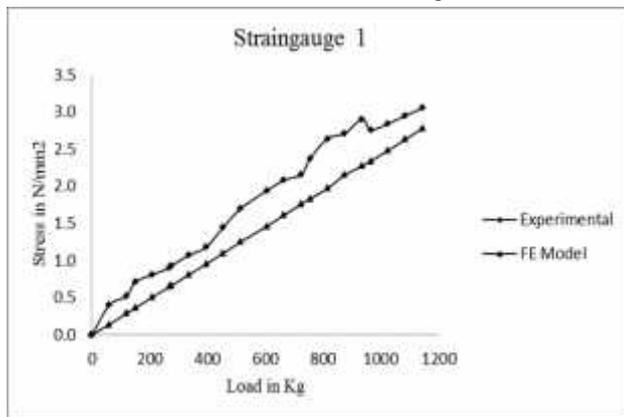
Fig.15. Stress at strain gauge 1 for FS I
