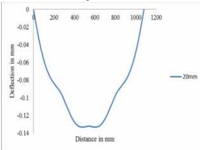
Fig.20. Deflection Curve for concrete funicular shell II
