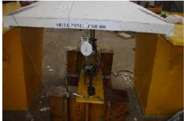
Fig.13. Location of dial gauges
