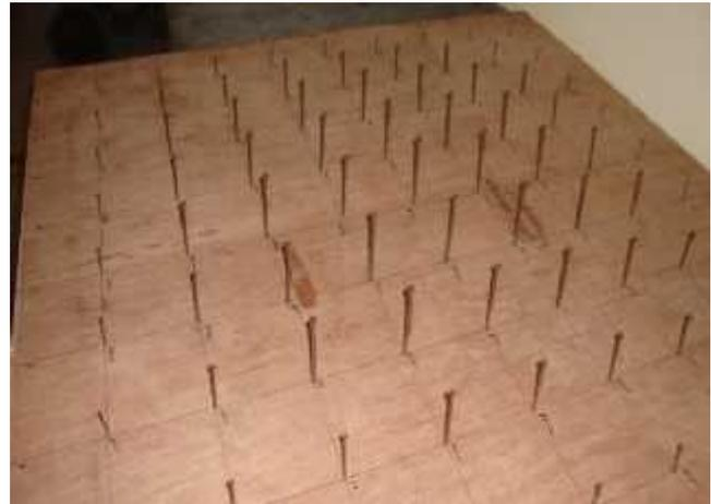
**Fig.3. Fixing shell coordinates**
