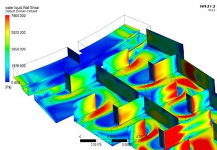
Fig 22: Wall shear at the Weir location
