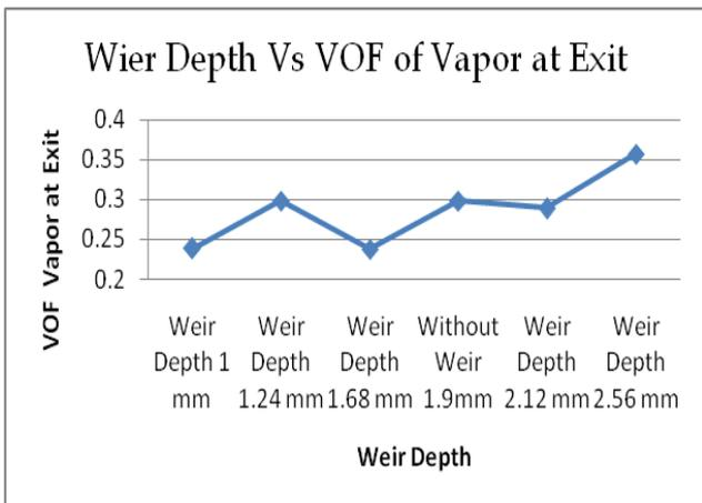
Fig 34: VOF water Vapor at Outlet Vs Weir Depth
