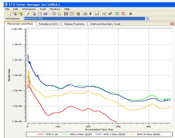
**Fig 7: CFX Solver Manager Convergence graph**
