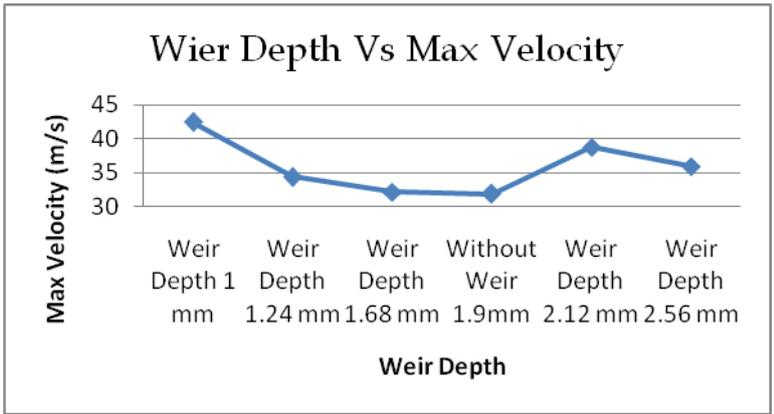
**Fig 32: Max. Velocity at Outlet Vs Weir Depth**
