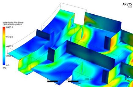
**Fig 31(A): Tortuous path Wall shear at the Weir location.**
