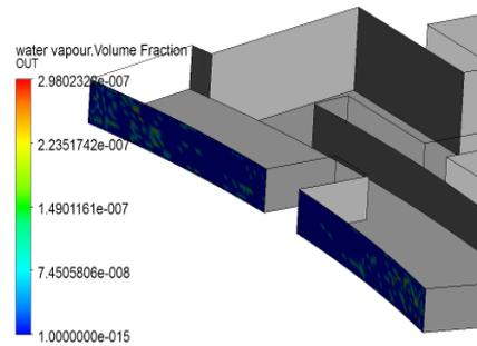
Fig 15: Water Vapor Volume fraction at Exit
