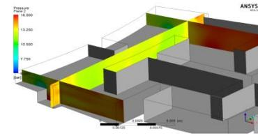
Fig 14: pressure Plot at the weir on a plane
