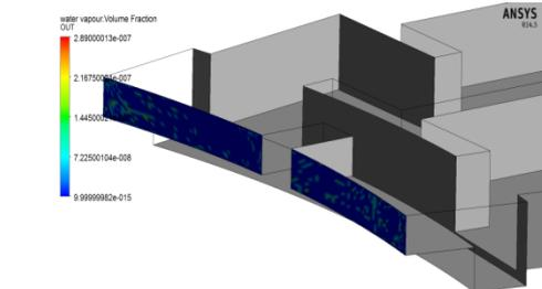
Fig 27: Water Vapor Volume fraction at Exit
