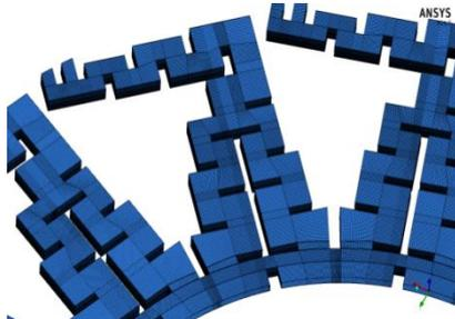
**Fig 6: Meshing of Disk (Details view)**
