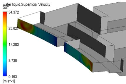
Fig 20: Velocity Plot at the exit
