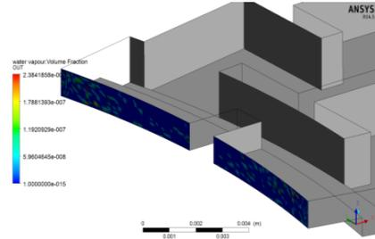
Fig 24: Water Vapor Volume fraction at Exit
