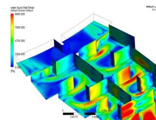
Fig 18: Tortuous path Wall shear at the Weir location
