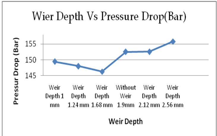
**Fig 31(B): Pressure Drop Vs Weir Depth**
