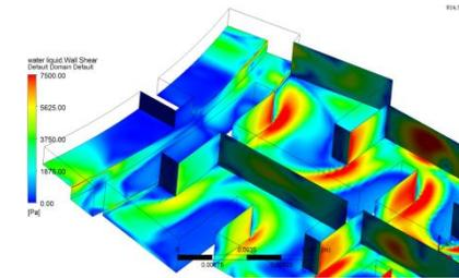
Fig 25: Wall shear at the Weir location
