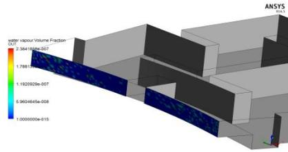
Fig 19: Water Vapor Volume fraction at Exit
