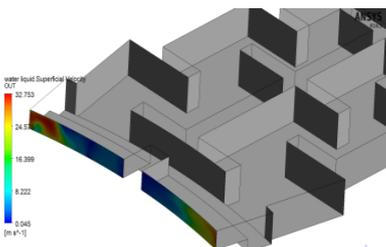
Fig 23: Tortuous Path Velocity Plot at the exit
