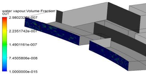
Fig 21: Water Vapor Volume fraction at Exit
