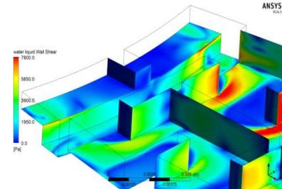
Fig 28: Wall shear at the Weir location
