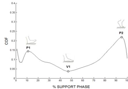
**Fig 1. Illustration of COF curve variables. Legend: COF: coefficient of friction; %SUPPORT PHASE: percent of support phase; P1 = RCOF1; V1 = Valley1; P2=RCOF2.**
