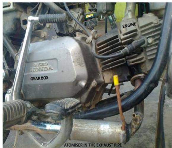
Fig 2 Atomizer in the exhaust manifold
