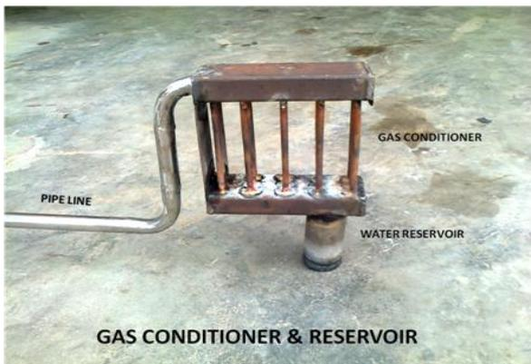
At the middle of the reservoir, there is a layer of urea has been located and this layer is help to the proper mixing of the water and the urea very well. And also there is a layer of filter located over the urea layer for filtering the Black Carbon (CB) or particulates matter (PM).
