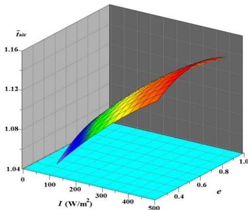
Fig.9. Surface of the response function at the air velocity  $v_{\infty}=0.2$  m/s
