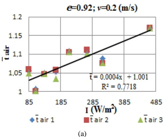
**Fig.7.** Experimentally found dependences of the relative air temperature  $\bar{t}_{air}$  on the irradiation intensity  $I, W/m^2$  at the air velocity over the irradiated area  $v_{\infty}=0.2 \text{ m/s}$  (a) Degree of blackness  $e=0.92$ ; (b) degree of blackness  $e=0.75$ ; (c) degree of blackness  $e=0.3$   $R^2$  – value of approximation reliability
