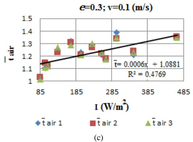
**Fig.5. Experimentally found dependences of the relative air temperature  $\bar{t}_{air}$  on the irradiation intensity  $I, W/m^2$  at the air velocity over the irradiated area  $v_{\infty} = 0.1$  m/s (a) Degree of blackness  $e = 0.92$ ; (b) degree of blackness  $e = 0.75$ ; (c) degree of blackness  $e = 0.3$   $R^2$  - value of approximation reliability**
