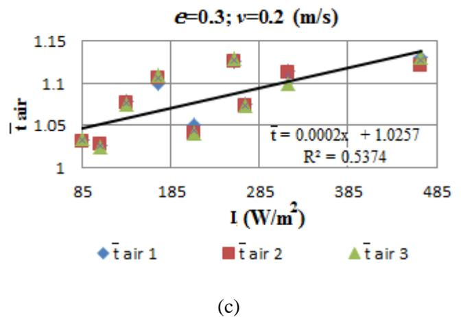
**Fig. 6.** Experimentally found dependences of the relative air temperature  $\bar{t}_{air}$  on the irradiation intensity  $I, W/m^2$  at the air velocity over the irradiated area  $v_{\infty}=0.15 \text{ m/s}$  (a) Degree of blackness  $e=0.92$ ; (b) degree of blackness  $e=0.75$ ; (c) degree of blackness  $e=0.3$   $R^2$  – value of approximation reliability
