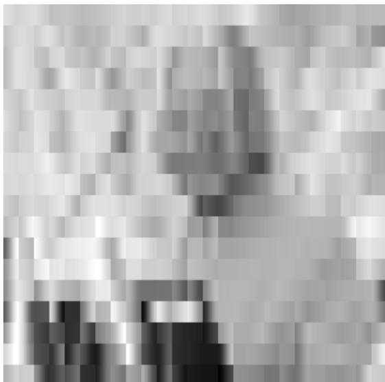
Fig. 4 Image after applying DCT compressed of 2 coefficients in 16x16 image sub-block.
