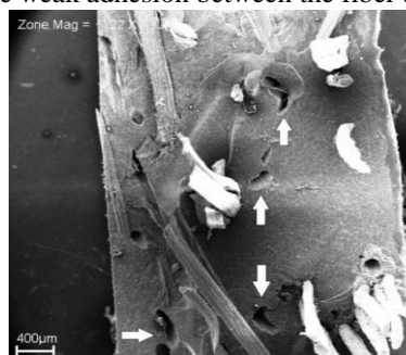
Fig. 5. Fracture surface of the polyester composite reinforced with 5 mm length sisal fibers. The white arrows indicate the fibers which pulled-out from the matrix.
